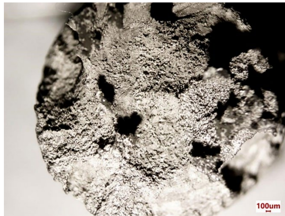
Fig. 3. The surface of NZ30K alloy additionally alloyed with Ag and clad with a layer of silver 200–300 nm thick after corrosion tests in Ringer–Locke solution.
